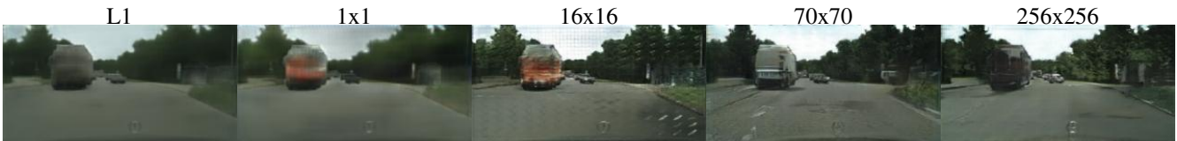
Figure 6: Patch size variations. Uncertainty in the output manifests itself differently for different loss functions. Uncertain regions become blurry and desaturated under L1. The 1x1 PixelGAN encourages greater color diversity but has no effect on spatial statistics. The 16x16 PatchGAN creates locally sharp results, but also leads to tiling artifacts beyond the scale it can observe. The 70x70 PatchGAN forces outputs that are sharp, even if incorrect, in both the spatial and spectral (colorfulness) dimensions. The full 256x256 ImageGAN produces results that are visually similar to the 70x70 PatchGAN, but somewhat lower quality according to our FCN-score metric (Table 2). Please see https://phillipi.github.io/pix2pix/ for additional examples.
